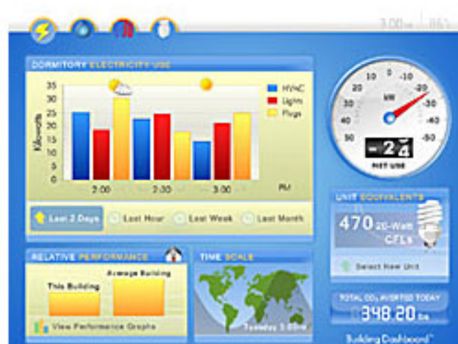
The Building Dashboard displays a building's energy consumption in real-time.
